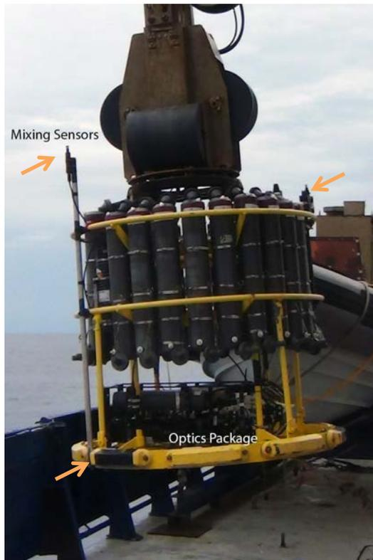
**Figure E-8: CTD cage with optic (lower package) and mixing sensors (probes attached to pipes at upper left under label, lower left, and upper right)**
