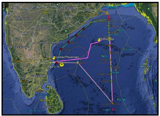
\*\*\* Green Line are Planned track, The Magenta line are the actual track, due to back to back low pressure systems in northern bay and worsening sea state, we bounded off the northern sections.
