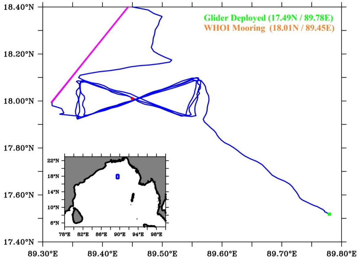
Figure 2. Deployment location (green circle) and track (blue line) of SG615 around WHOI (18.01°N, 89.45°E) mooring (Red circle). The approximate track of dive 41-59 is marked in pink color.
