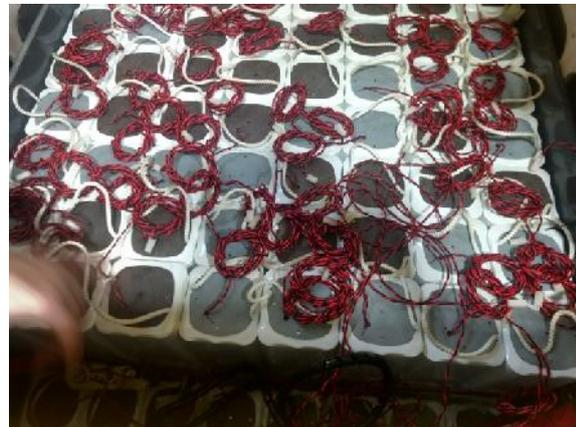
Halo section (left) and well of the INCOIS mooring with fully assembled 80 Battery packs
