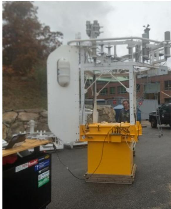
ASIMET Data Logger in the Buoy well and Buoy under Spin test.
