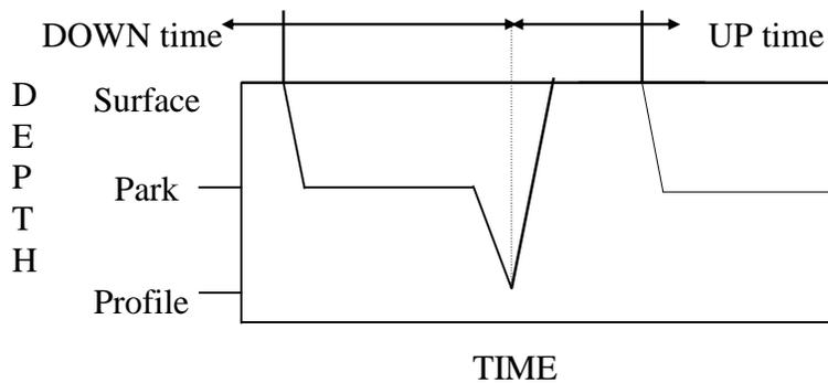
Parameter **PD** determines the frequency of deep profiles.
