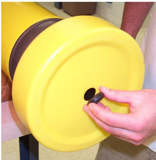
2. The minimum internal temperature of the float is - 2.0 °C. If necessary, let float warm indoors before proceeding.
