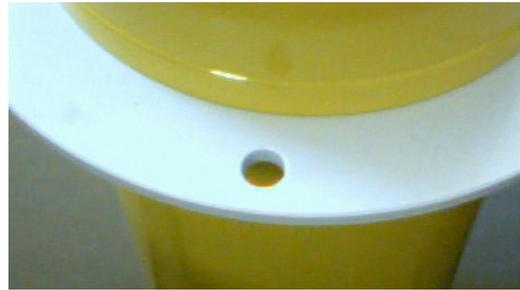
It may take several minutes for the cowling to fully flood with water and the float may drift at an angle or even rest on its side during this period. This is normal behavior and not a cause for concern.
