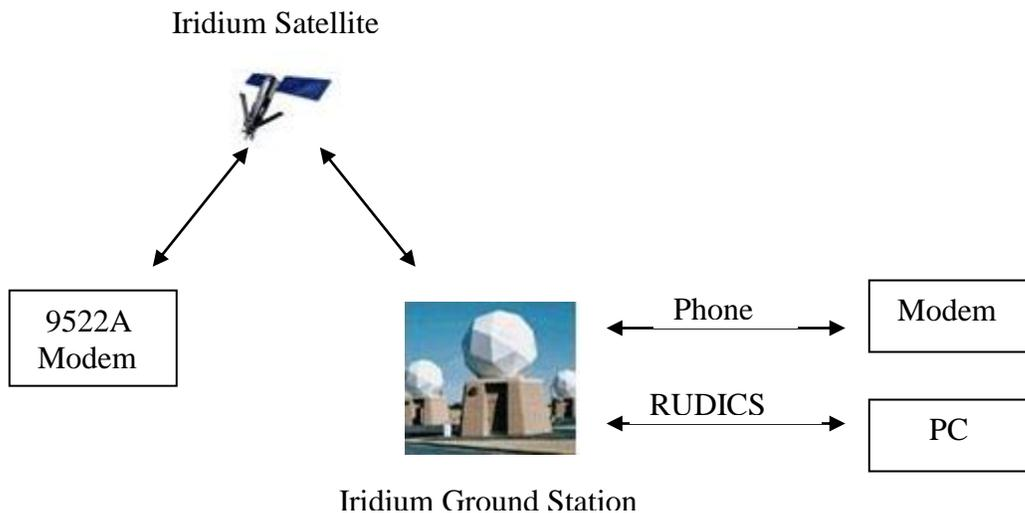
For modem-to-modem communications (without RUDICS) you will need independent primary and alternate host servers, each with a modem connected to the phone system to receive the calls and data from the float. A full description of this equipment and software is beyond the scope of this manual. However, Teledyne Webb Research makes regular use of U.S. Robotics external modems, Model USR3453C, Courier™ 56K Business Modem.
