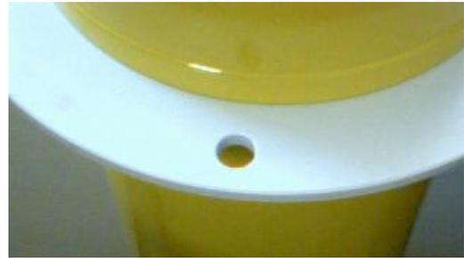
It may take several minutes for the cowling protecting the bladder to fully flood with water and the float may drift at an angle or even rest on its side during this period. This is normal behavior and not a cause for concern.
