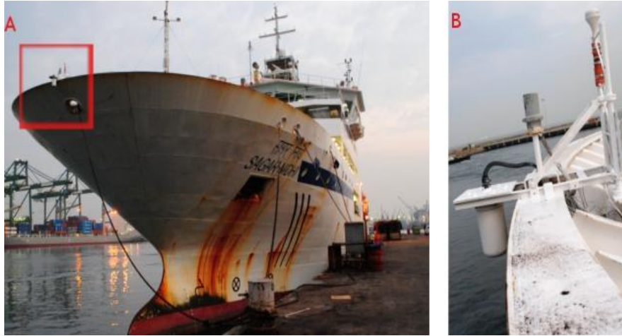
Wave Height Meter Installed onboard ORV Sagar Nidhi
