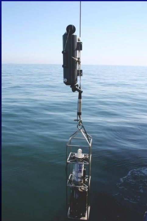
Hydrocast using a Niskin bottle and portable CTD
