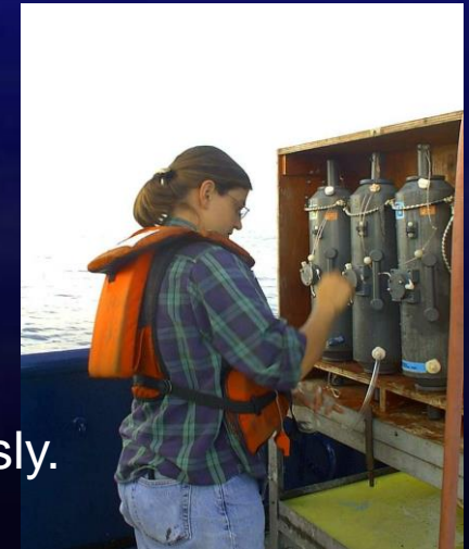
An Oceanographer sub-sampling sea water from Niskin bottles
