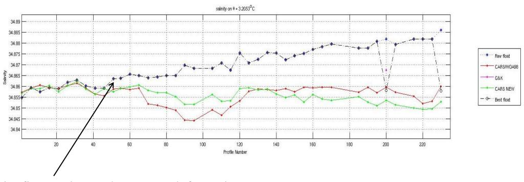
This float is observed to posses drift in salinity starting from cycle 44 onwards
