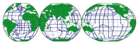
Positions of XBT temperature profiles from merchant ships in 2002. Note poor coverage in southern hemisphere
