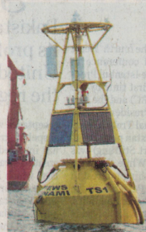
A buoy that is a part of a tsunami warning system.
