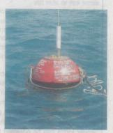
Wave rider buoys are being used for real time data. – PHOTO: N. RAJESH
