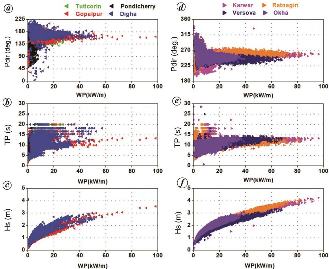
**Figure 5.** Scatter plots of wave parameters ( $P_{dir}$ ,  $T_p$ ,  $H_s$ ) with wave power (WP) off the (a–c) east coastal and (d–f) west coastal areas of India during SM.
