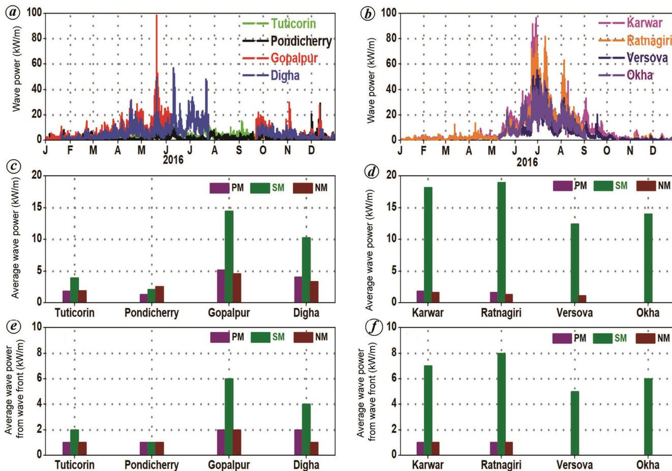
**Figure 4.** Annual time series of wave power along the (a) east and (b) west coastal areas of India. c, d, Average wave power off the (c) east and (d) west coastal areas. Average wave power from wavefront off the (e) east and (f) west coastal areas.
