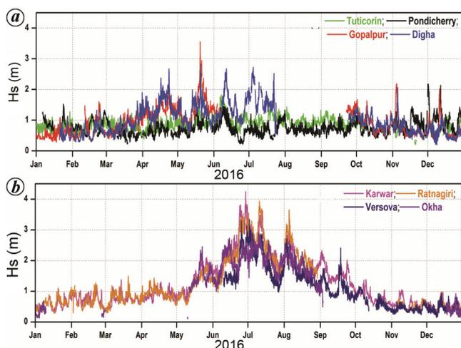
**Figure 2.** Time series plots of significant wave height in the (a) east and (b) west coasts of India.
