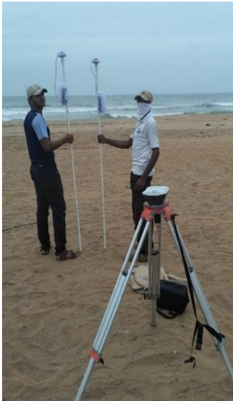
Figure 6. Tracking of shoreline position using the Emlid Reach RTK-GPS at selected areas.
