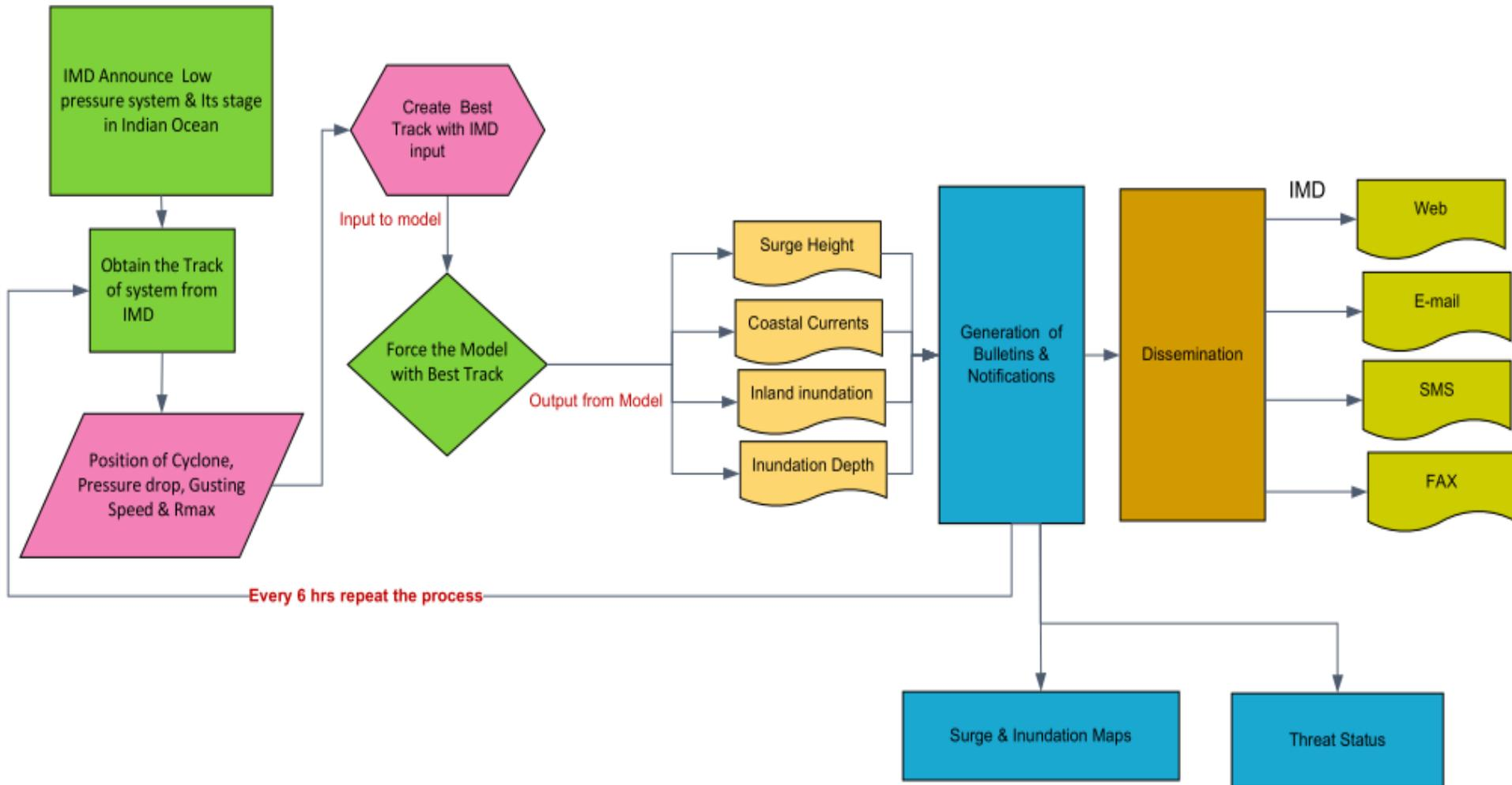
**Figure:** Standard Operating Procedure of Storm Surge Early Warning
