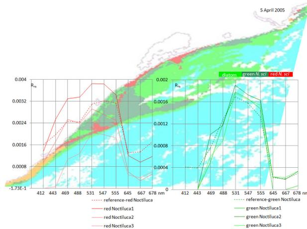
Figure 6. Reference  $R_{rs}$  spectra (discrete) for red and green *Noctiluca* and for the pixels for these species from 5 April 2005 image
