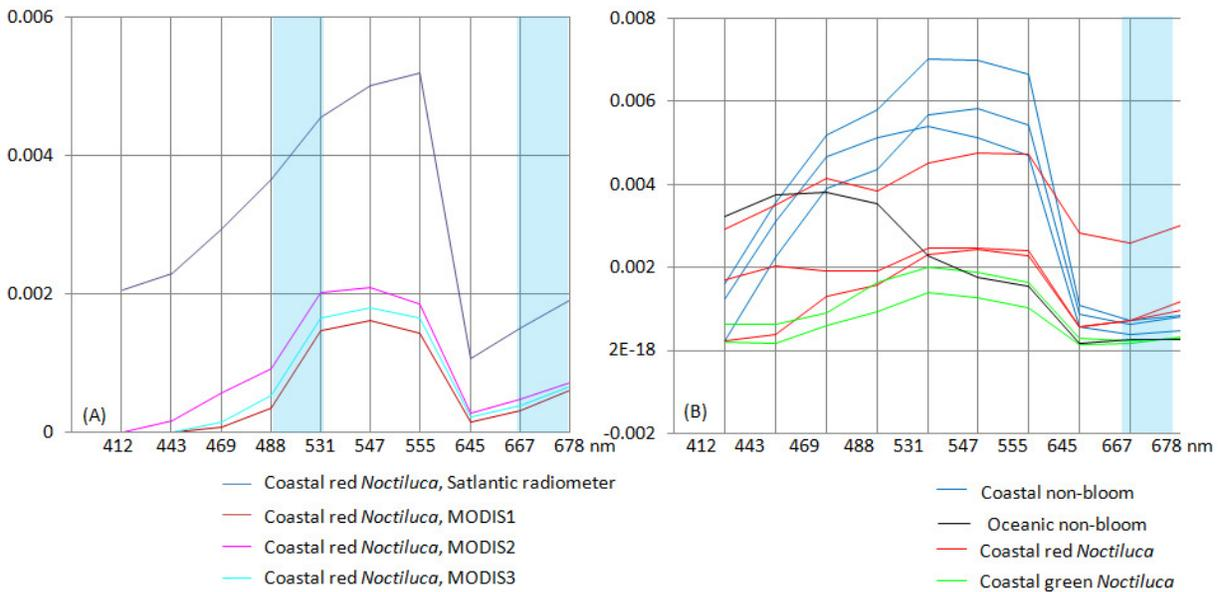
Figure 3. (A) Discrete  $R_{rs}$  spectra corresponding to MODIS bands using the radiometer (B) Typical  $R_{rs}$  spectra for red, green *Noctiluca* and non-bloom waters (coastal and oceanic)
