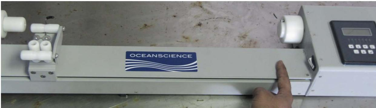
**Figure 2: Tail spool Re-winder, indicating the stopping terminal of spectra line.**
