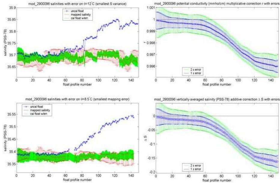
Figure 6: Calibration using WOA alone
